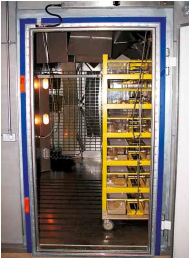
View into an exposure chamber with animal cage racks
